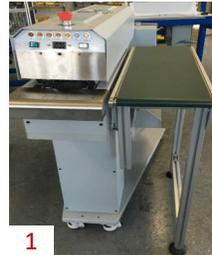
Conventional conveyor powered or unpowered extension tables to support long heavy harness
